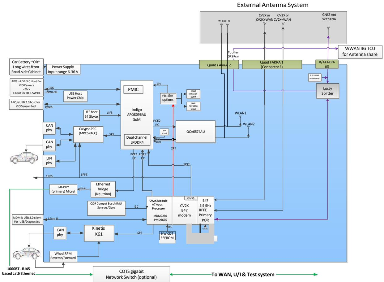
Figure 2-3 CV2X Development Platform high-level block diagram
