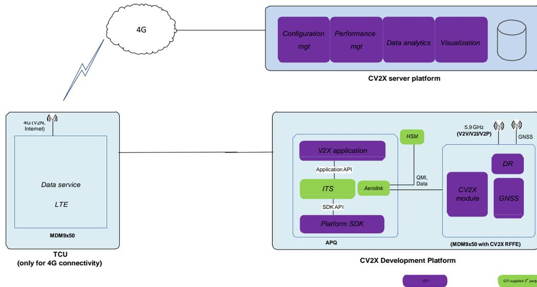
Figure 2-2 CV2X platform system architecture
