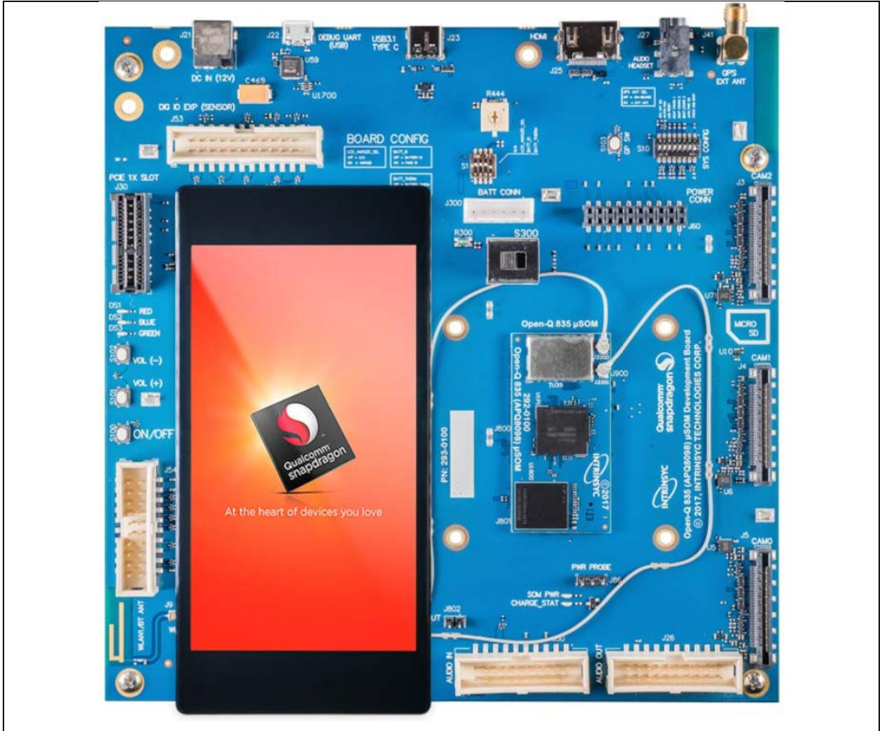
Figure 1 Assembled Open-Q 835  $\mu$ SOM Development Kit
