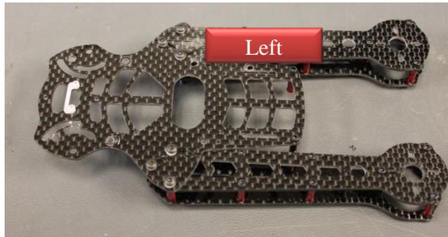
Figure 6 Attach each arm to the bottom plate
